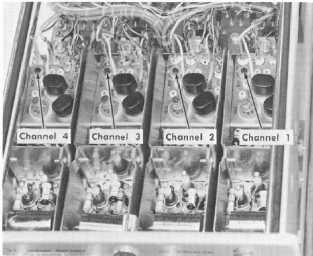
(B) Location of the PREAMP GAIN adjustments R77 for each channel. Bottom center-portion view; securing rod removed.
